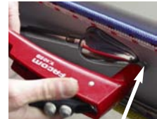
fixing a safety rivet
